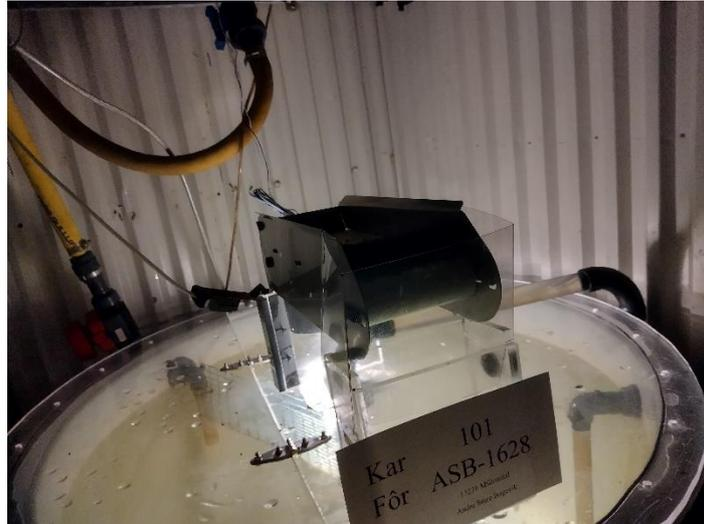
Figure 12. The fish were feed with a belt feeder. Each feeder was labelled, to reduce chances of tanks mistakenly being feed the wrong feed.
